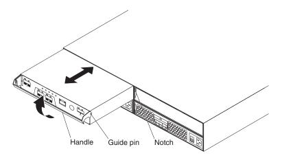
Figure 52. Removing a controller
